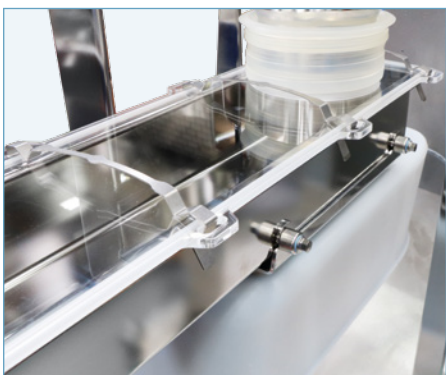
Special quick-release clamps hold the cover on the tray.
