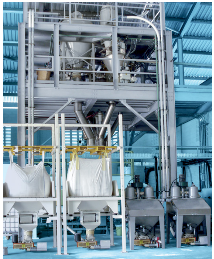
› PVC COMPOUNDING SYSTEM – COMPLETE SYSTEM AND CONTROLS DESIGNED BY COPERION K-TRON IN FULL COOPERATION WITH CUSTOMER TO ENSURE A CONSISTENT AND RELIABLE END PRODUCT.
