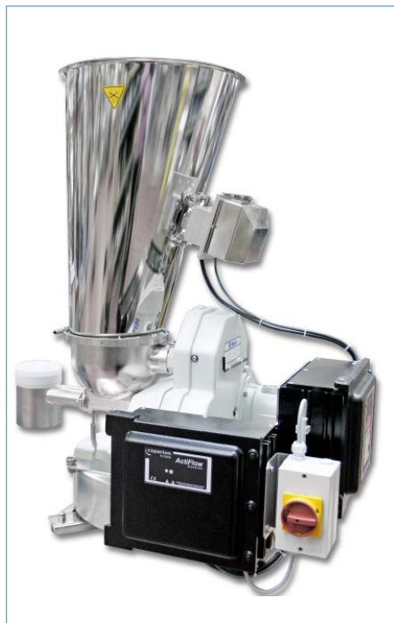
Figure 6: Coperion K-Tron twin screw feeder with ActiFlow™ bulk solid activator. ActiFlow eliminates headroom concerns, reduces cleaning and product changeover time and in turn lowers overall production labor cost.
