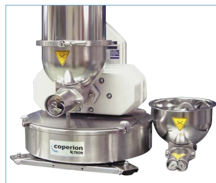
Figure 7: Coperion K-Tron Quick-Change Feeder QC with exchangeable feeder module.
