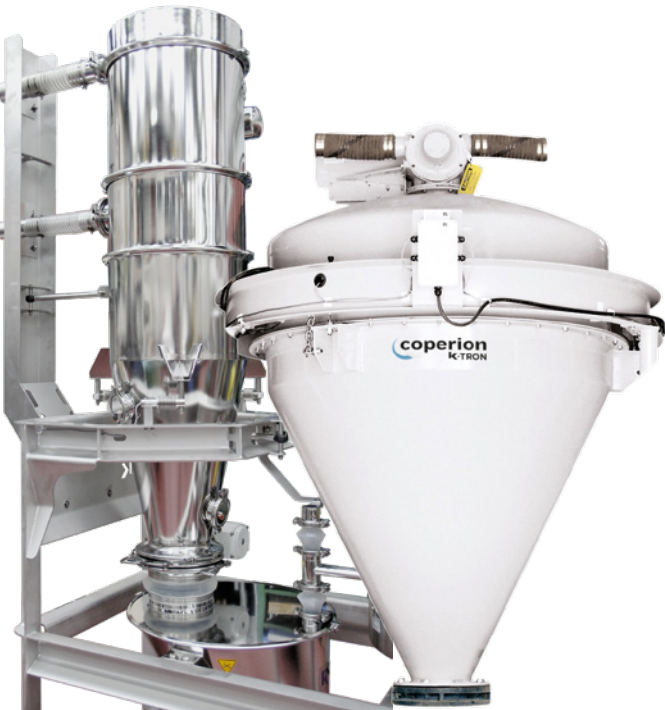
Batch weigh receivers and scale hoppers are often used with diverter valves
