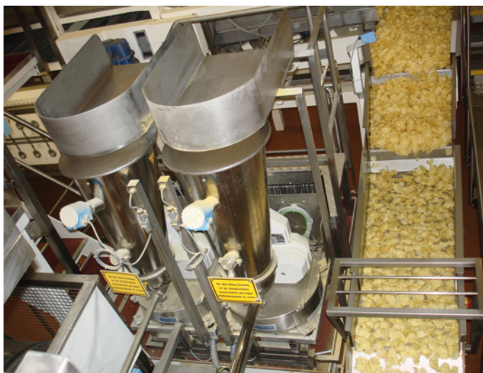
Coperion K-Tron LIW feeders delivering seasonings in coating process
