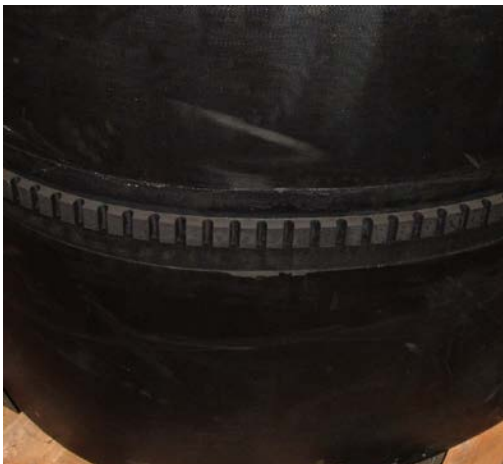
Molded V-guide maintains proper belt tracking and alignment
