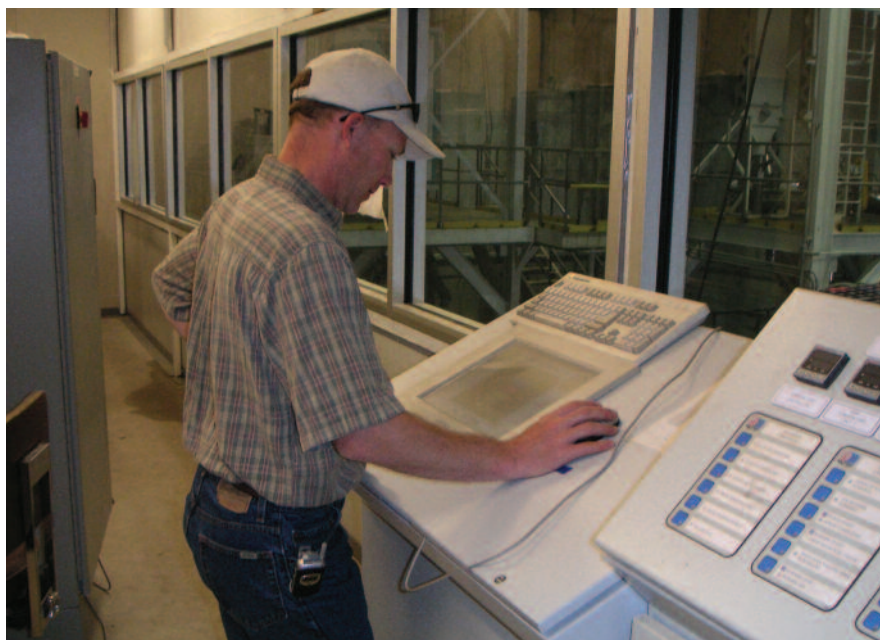
An operator controls the corn flour production process using a color touchscreen operator interface installed in a central control room that overlooks the facility's processing lines.
