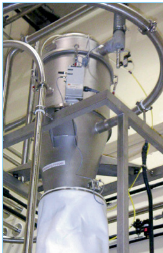
Series 2400 receiver conveying salt
