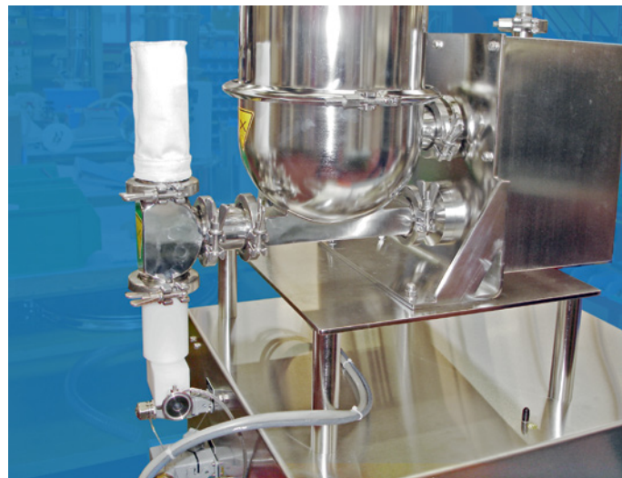
Volumetric pharmaceutical feeder with gas venturi on outlet
