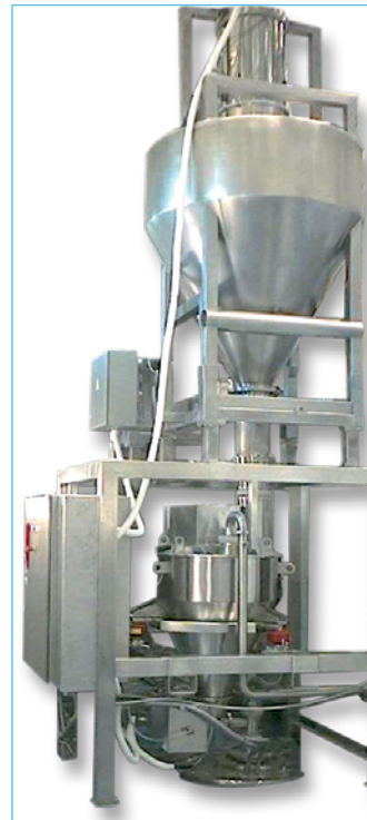
Coperion K-Tron P-Series pneumatic receiver and LIW feeder with IBC dispensary station
