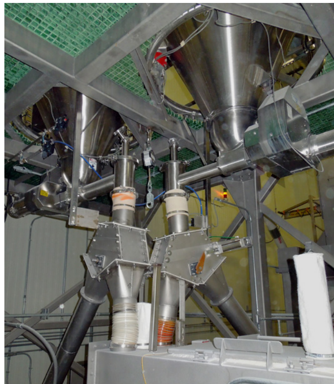
Photo 1: Coperion K-Tron Loss in Weight Feeders Feeding Spice Ingredients to Continuous Mixer
