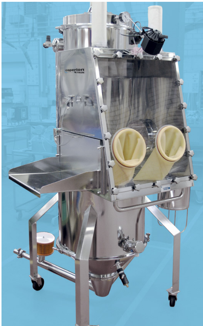
Sanitary bag dump station with integrated glovebox for conveying Probiotics directly to a P-Series vacuum receiver
