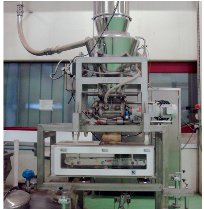
Smart Weigh Belt feeder shown with vacuum receiver, buffer hopper and rotary pre-feeder.
