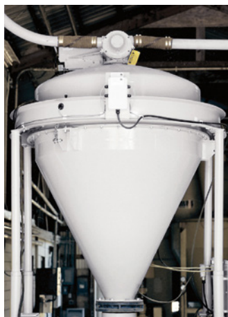
Scale hopper with diverter valve at top
