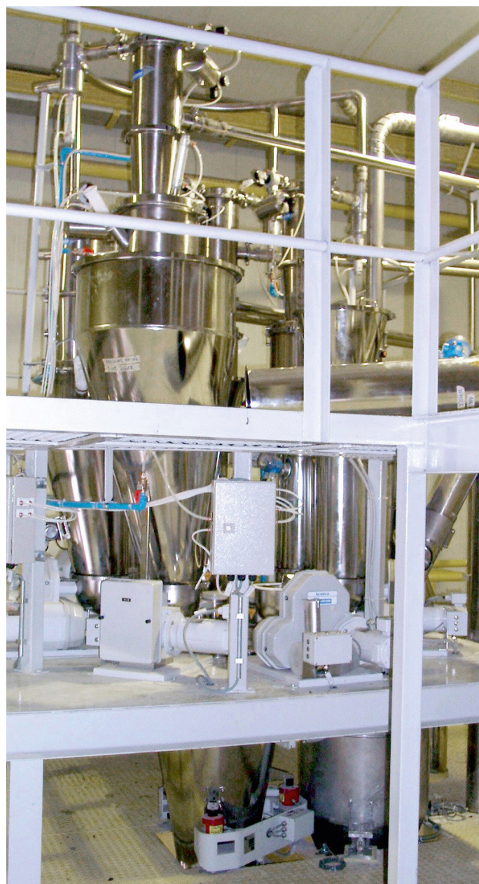
Gain-in-weight batching station for a bakery installation in Indonesia.
