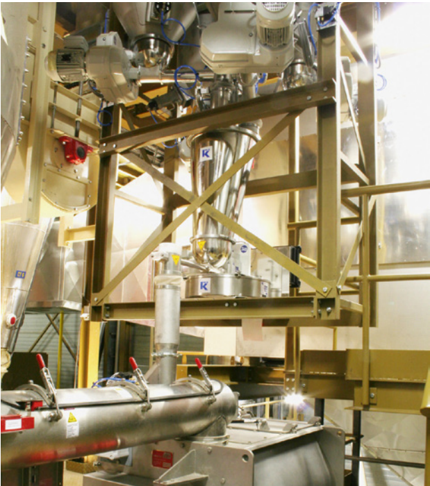
Loss-in-weight screw feeder feeding into a mixer
