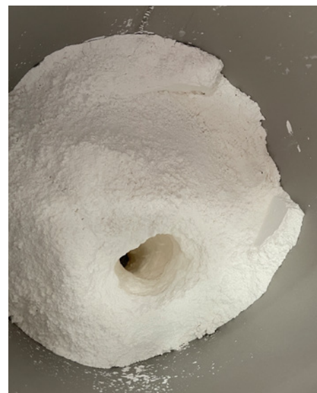
Figure 9 - Cohesive powders often do not flow well, forming ratholes in a hopper.
